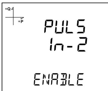
1. Press the SET button while SETUP-PULSE IN is displayed.
