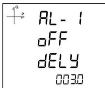
1. After entering a hysteresis value, press the UP button to find the Alarm On Delay menu.
