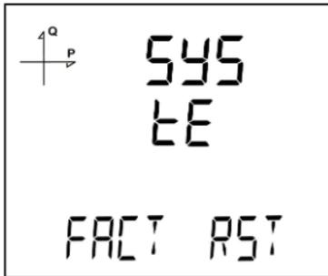
1. To reset the device to factory settings, press the SET button while "FACT RST" is displayed.
