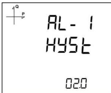
1. While Alarm Enable is selected, find Alarm Hyst menu with UP/DOWN buttons.
