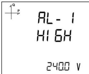
1. While Alarm Enable is selected, find Alarm High menu with UP/DOWN buttons.
