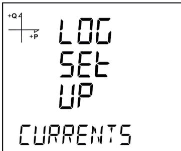
1. Press the SET button while Log Setup-Currents is displayed.
