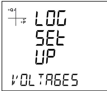
1. Press the SET button while Log Setup-Voltages is displayed.
