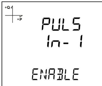
1. Press the SET button while SETUP-PULSE IN is displayed.
