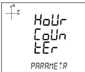
The device can count the time when a selected parameter exceeds or falls below an adjusted limit value. This feature is explained in this section.
