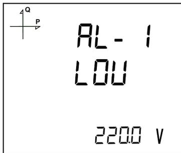
1. While Alarm Enable is selected, find Alarm Low menu with UP/DOWN buttons.
