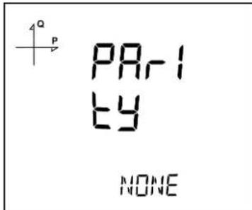
Communication parity of the device can be set as Odd, Even or None.
