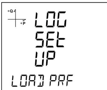
1. Press the SET button while Log Setup-Load Profile is displayed.
