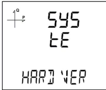
The device's hardware and software version can be displayed under this menu:
