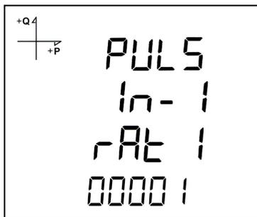
1. Press UP button while PULSE IN-1 Enable is displayed.
