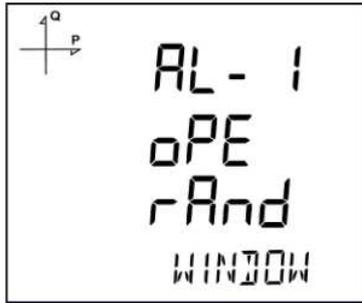
1. While AL-1 OPE RAND is displayed, press the SET button to select the alarm operation type.
