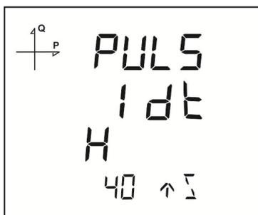
For devices with pulse counting feature, the minimum time necessary for the pulse counting can be selected from following options:
