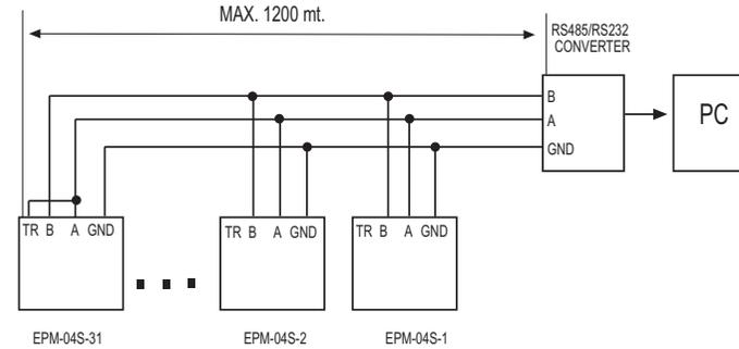
MAX. 247 DEVICES CAN BE CONNECTED AT SAME LINE BY USING REPEATER.
