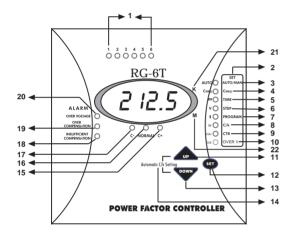
On the front panel of RG-6T, there are warning lights, display and 3 buttons for settings.
